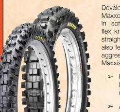
Developed for use in the GNCC, the Maxxcross SI delivers excellent traction in soft/intermediate conditions. Its antiflex knob bridges on side lugs offer solid straight-line stability. The Maxxcross SI also features an enhanced grip to allow for aggressive cornering. The SI is proof that Maxxis takes performance to the next level.
