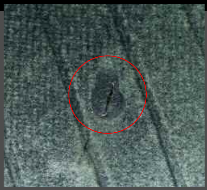
Puncture - Normally, the only evidence of a puncture will be a cut that extends from the tread of the tire through the inner liner.
