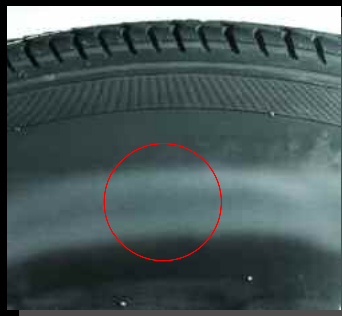
Under-Inflated Tire - An abrasion may run around the circumference of the tire and wrinkles may be observed in the inner liner.
