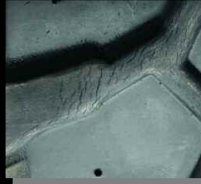
Cracking Between Tread
