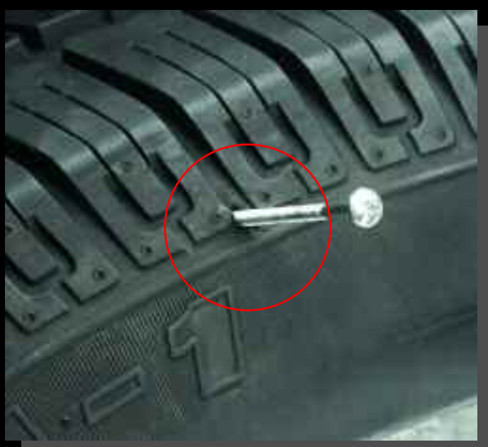
Puncture - Normally, the only evidence of a puncture will be a cut that extends from the tread of the tire through the inner liner.
