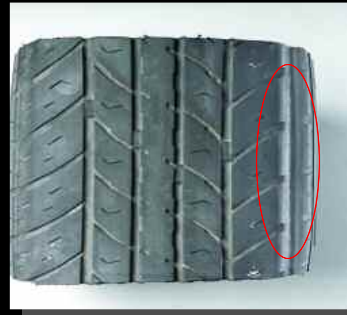
Shoulder Separation - A groove worn in the shoulder of the tire is usually evidence of separation.
