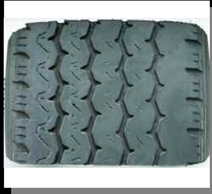
Rapid Shoulder Wear
