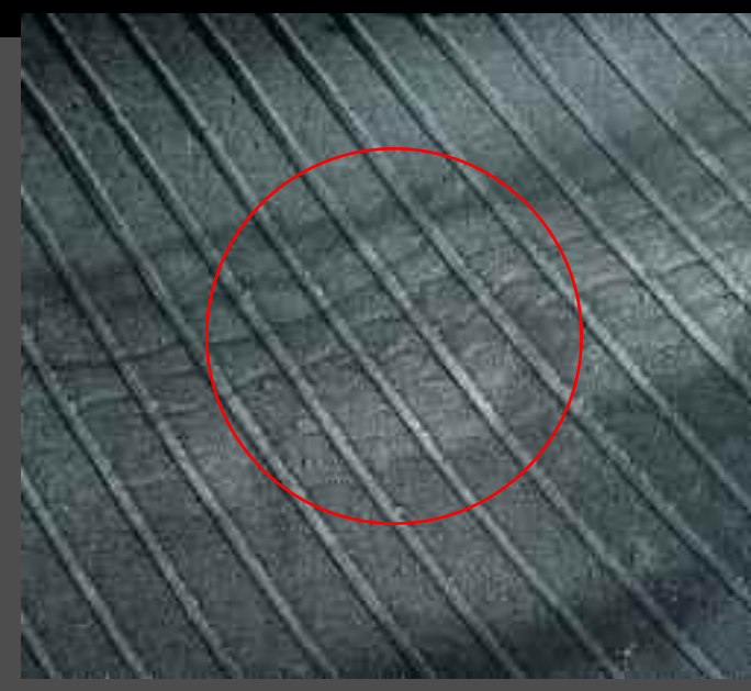
Under-Inflated Tire - An abrasion may run around the circumference of the tire and wrinkles may be observed in the inner liner.
