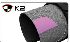
**ZK:** our lightest and most supple under-tread puncture protection layer
